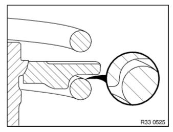
• Check the position of the spring plate in the coil spring at the top and bottom and, if necessary, correct it.
