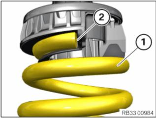
• Position the top spring pad on the coil spring (1) in such a way that the coil spring end (2) is on form-fit contact with the top spring pad.
