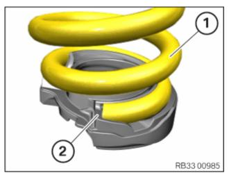
Position the coil spring (1) in such a way that the lower coil spring end is in form-fit contact with the lower spring pad (2).
