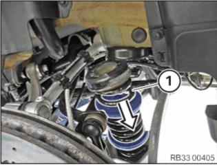
• Insert and position the coil spring (1) from above in the arrow direction.
