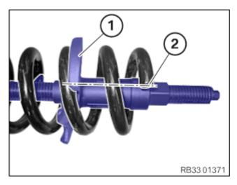
• Align the lower spring plate (1) with the opening for the lower coil spring end (2).
