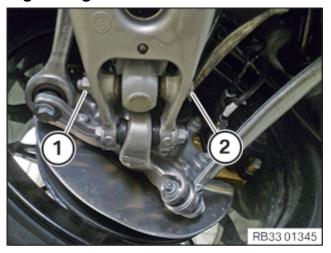
• Slacken the nut (1) by a turn and tighten it. Provide counter support to screw (2) in the process.
