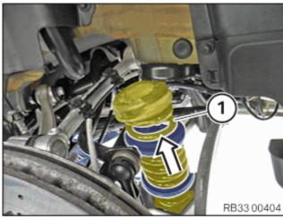
• Guide out and remove coil spring (1) upwards in the arrow direction.
