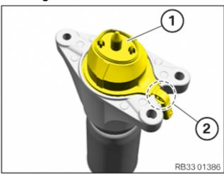
• Check the position of the centering cap (1) and the adapter lead (2), correct if necessary.
