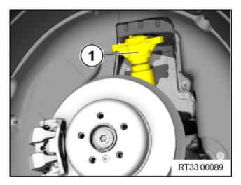
• Compress the shock absorber (1) and feed it into the wheel well.
