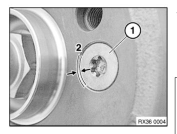
Check if the mounting bolt (1) has been fitted correctly for the brake disk.
