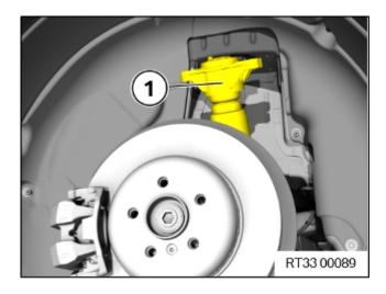
Compress the shock absorber (1), feed it out and remove it.
